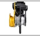
Main faceted sheave with single-direction rotation provides excellent efficiency when hauling and additional braking when lowering heavy loads.
